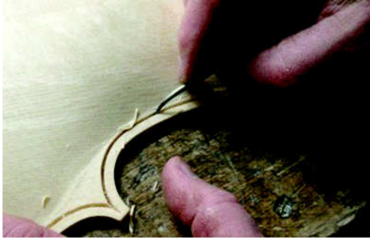
Figure 1: Cutting the purfling groove. (Picture from the internet)
