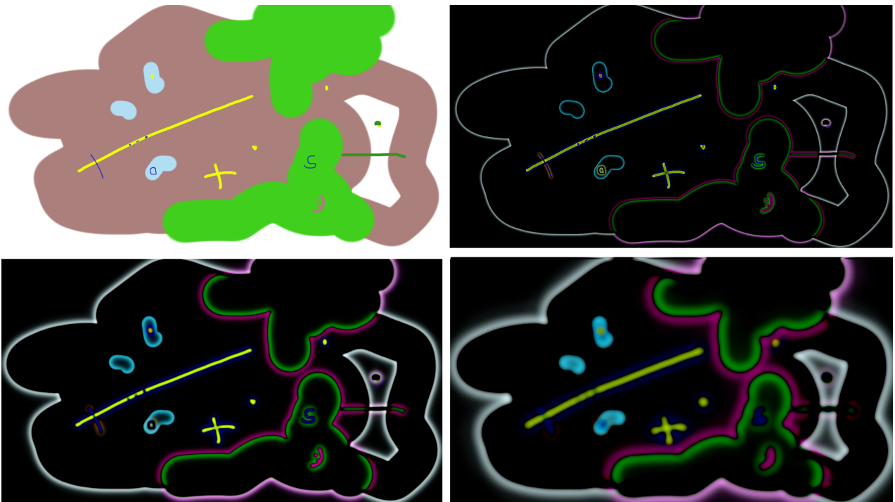
Figure 17: A demonstration image and three derived images by applying DoG with radii 1:2, 3:5 and 8:13.
