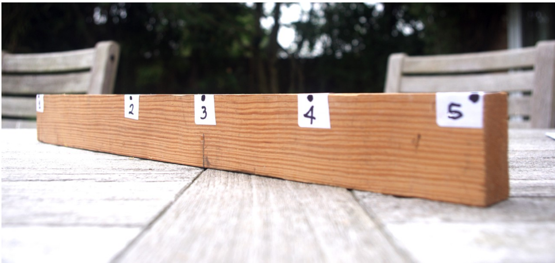
Figure 3: Five point objects on a wooden bar at mid-lens height. They are 10 or 20 cm apart.
