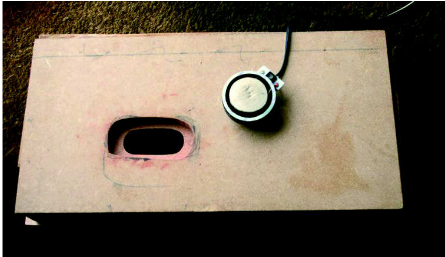
Figure 1: The wooden box, clad in MDF, with a cut-out around the aperture (61 by 28 mm) in the top plywood plate. The electromagnetic exciter has been placed on top, though it was applied to the bottom plate of 2·91 mm thick plywood. Not my finest piece of woodwork!
