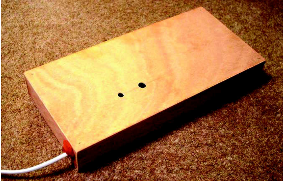
Figure 29: Plywood Box A with 9 and 11 mm holes, and cable for internal electret microphone.
