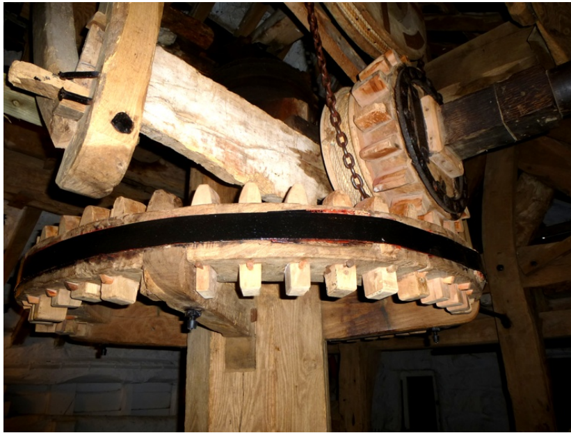
Figure 14: Wooden peg teeth in the crown and pinion gears at the top of the upright shaft at Stretton water mill, Cheshire.
